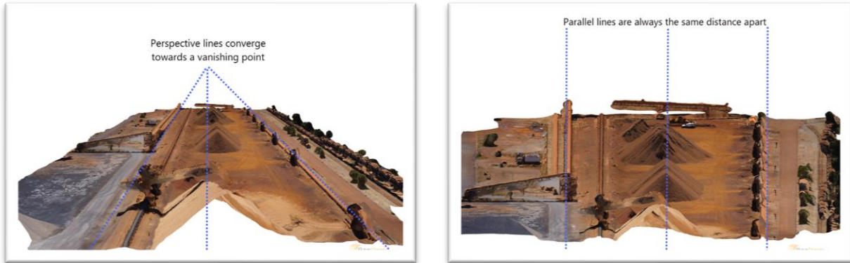
Figure 3 Camera with a perspective view (left) and parallel view (right)
