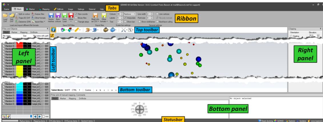
Figure 1: The GEM4D interface objects naming convention
