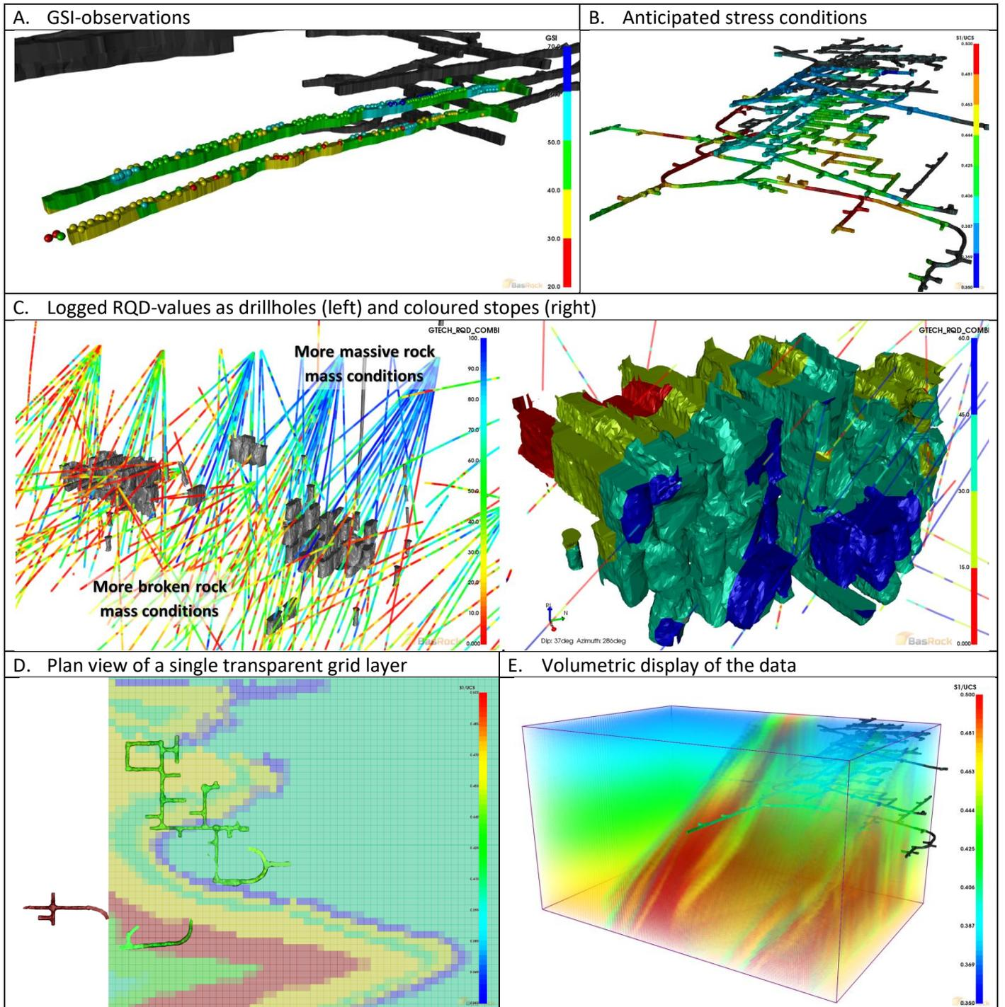
Figure 4: Different ways to visualise geotechnical data and block models
