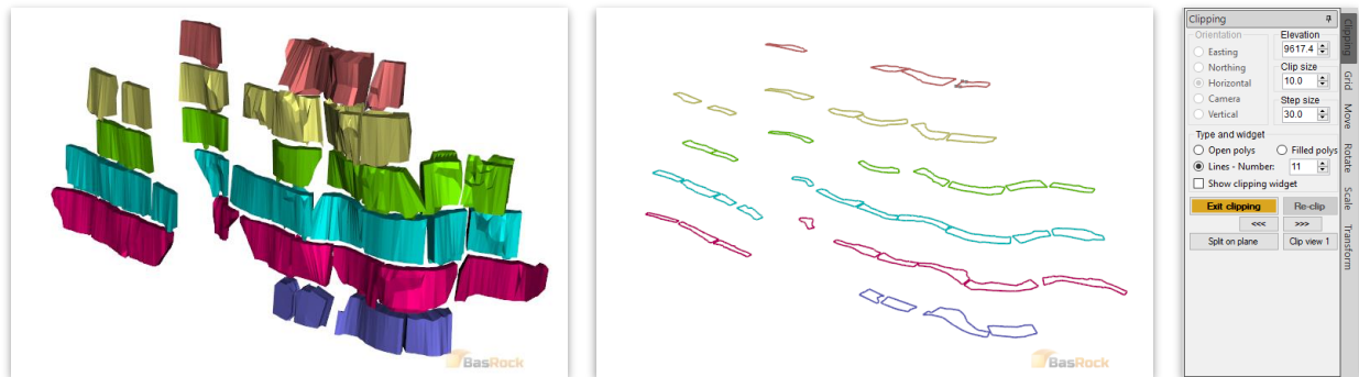
Figure 2 Original meshes (left), lines clipping (middle), and clipping settings (right)
